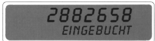
When registration is over, the CMT shows the subscriber number which it has extracted from signalling
