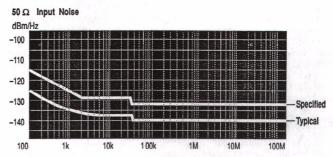
Specified for swept spectrum mode, with 50  $\Omega$  input range set to  $-20 \mbox{dBm}$  and low-distortion mode off.
