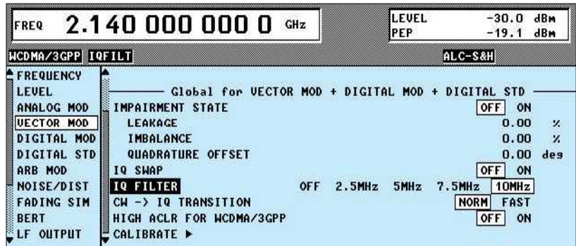
FIG 3: Four different I/Q filters allow ACLR performance of single-carrier to four-carrier WCDMA signals to be optimized
