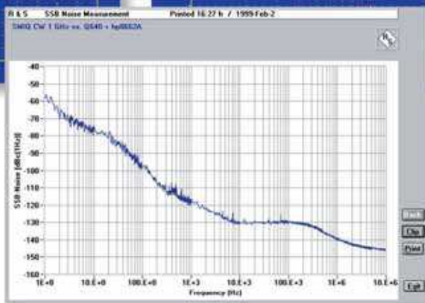
Typical SSB phase noise at f_c=1 GHz
